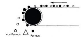
Material is carried along the conveyor. The magnetic head pulley holds ferrous metal to it's surface allowing the 'cleaned' product to follow its normal trajectory. Ferrous metal is held to the belt surface and carried round and under the pulley where it then discharges
